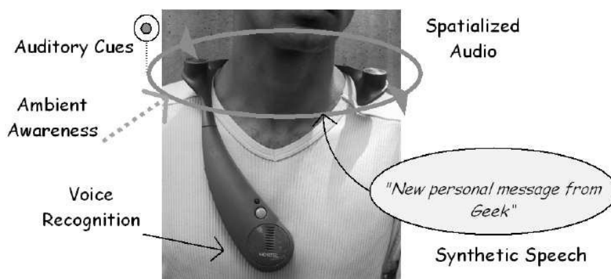
Figure 2.5: Description of the Nomadic Radio system with the SoundBeam Neckset audio device
